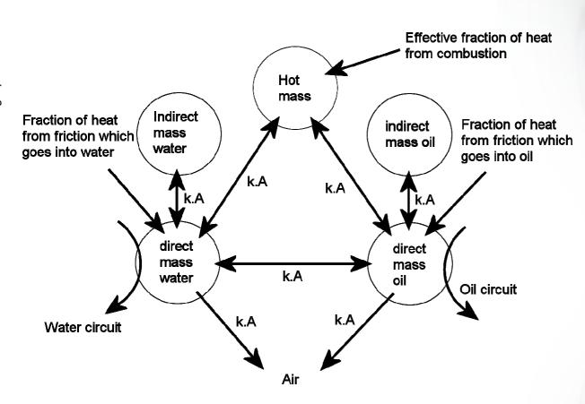
In the 5-mass model the hot pistons are included as an additional mass.
